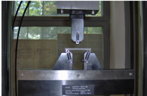
Fig 2. The universal machine LFV 25 HH WALTER-BAI
